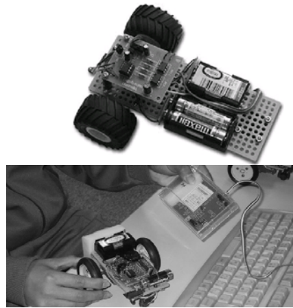
Figure 7. A robotic car, sample program and transferring programs using an infrared ray
